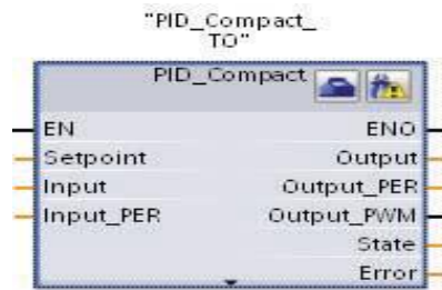
Fig. 7. PID on Siemens S7-1200 PLC [9].
