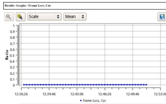
Fig. 9. Graphic of Frame Loss Measurement on Jakarta – Bogor Main Link.
