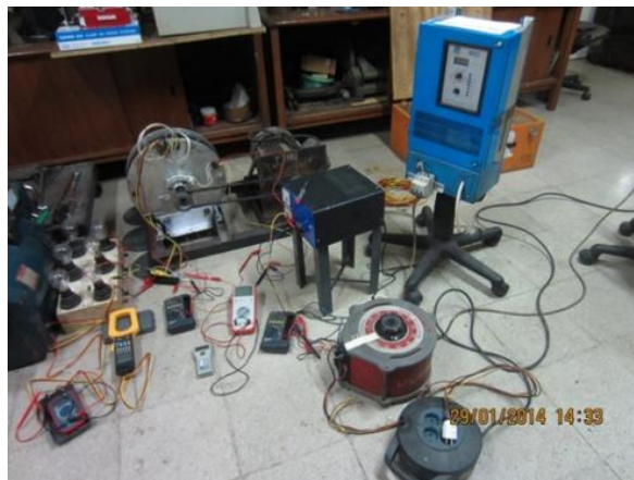
Fig. 7. The equipment utilized in the test of FWR generator.
