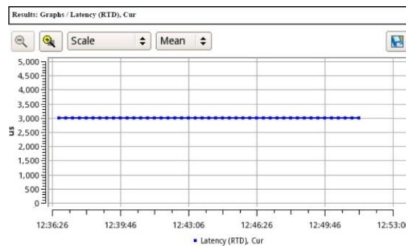
Fig. 11. Graphic of Latency Measurement of Jakarta – Bogor Main Link.
