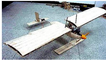
Fig. 16. Hybrid propulsion system for air-water drone developed by Nanchang Hangkong University
