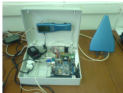
Figure 4: The EMF monitoring node contains a mini-ITX and a low cost EMF monitor (Spectran 60X0 analyzer, which can measure up to 7 GHz).
