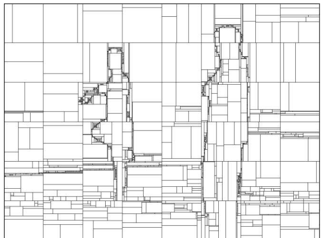
Figure 6. Example of PS obtained for 0.05 \text{bpp} (test sequence Ballet). There are 1780 blocks in the scheme.
