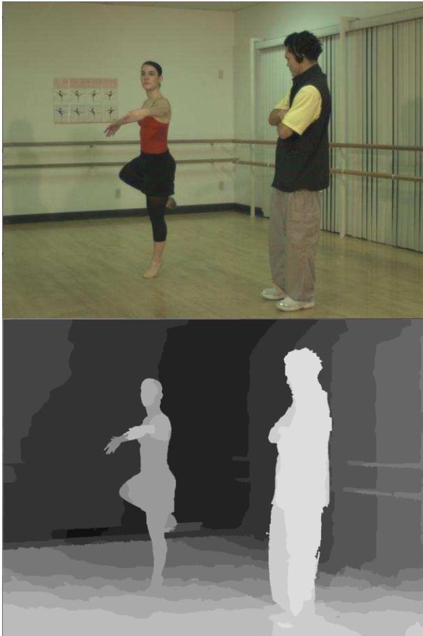
Figure 3. The test sequence Ballet, cam3, frame 98. Top: RGB component of the frame; bottom: corresponding depth map.
