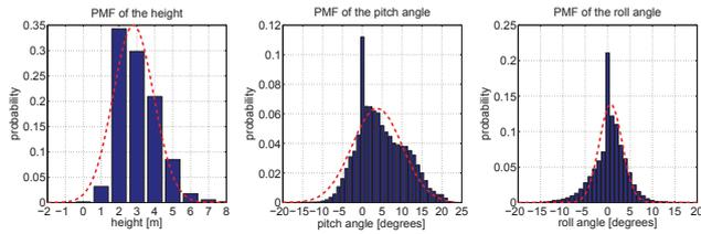
**Figure 1:** Probability Mass Functions of the height  $h_t$ , pitch angle  $\theta$  and roll angle  $\gamma$  of the UAV during the trials; the red dotted line represents the Gaussian fitting of the collected data, in blue.
