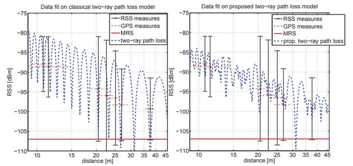
**Figure 2:** Empirical data fit on two-ray path loss model (left plot) and on the proposed one,  $\tilde{P}L$  (right plot).
