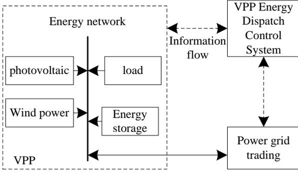
**Figure 1.** Schematic diagram of the operational structure of the virtual power plant
