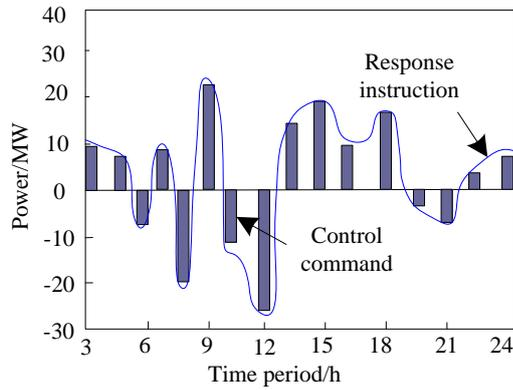
**Figure 4.** Actual Dispatch Control Instruction Response Results of Virtual Power Plant
