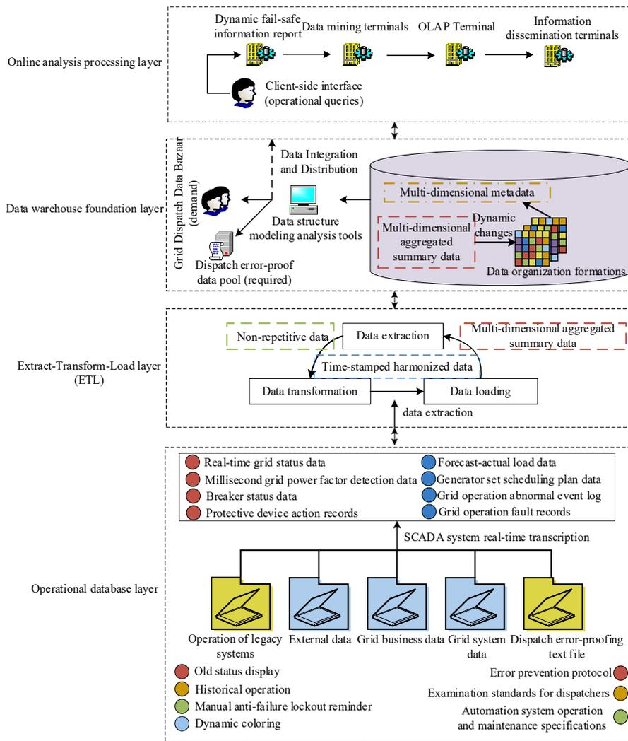
Figure 1. Layered structure of grid dispatch error-proof data warehouse
