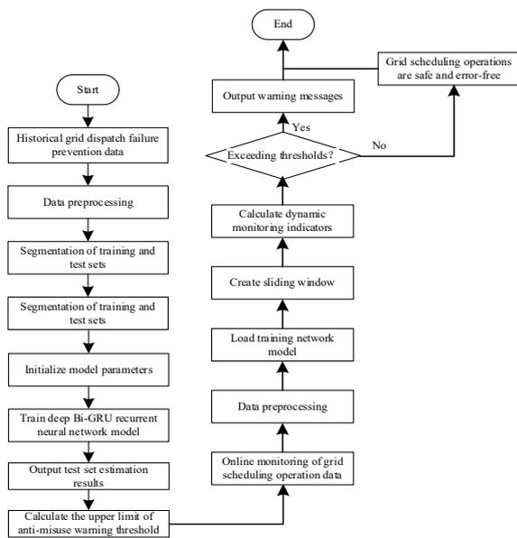
Figure 4. Grid dispatching anti-misoperation warning based on anti-misoperation state prediction model
