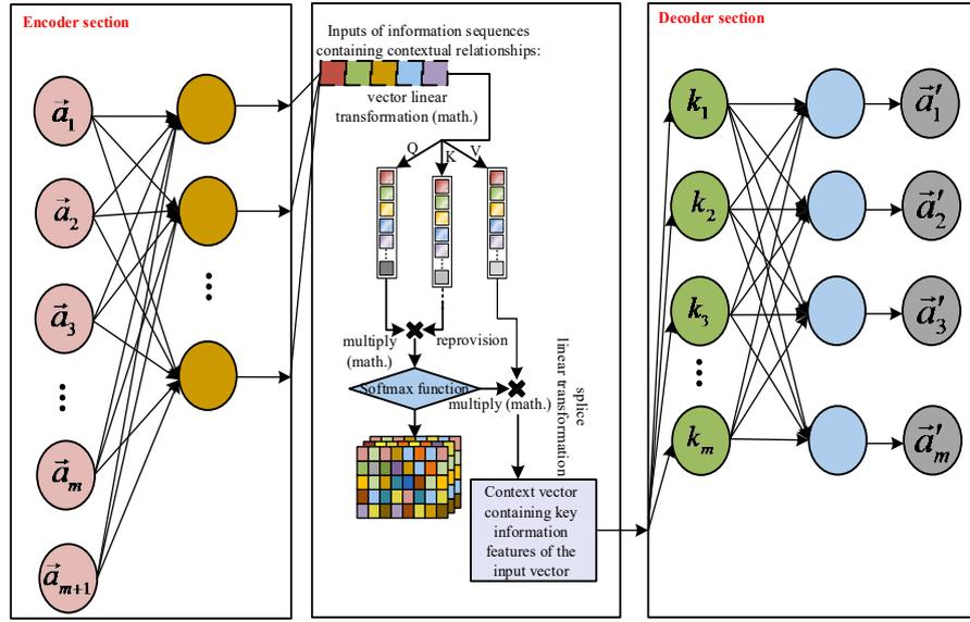
Figure 3. Self-encoder main structure
