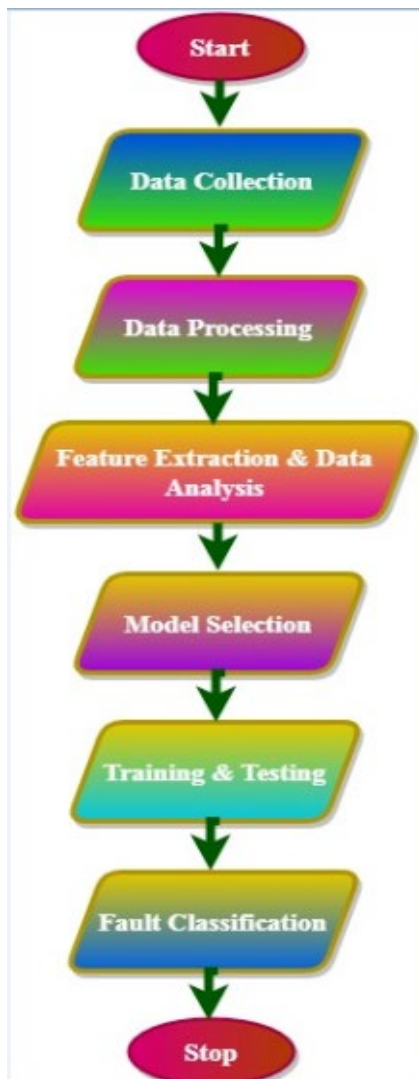
Figure 2. Solar PV fault detection and classification Flowchart
