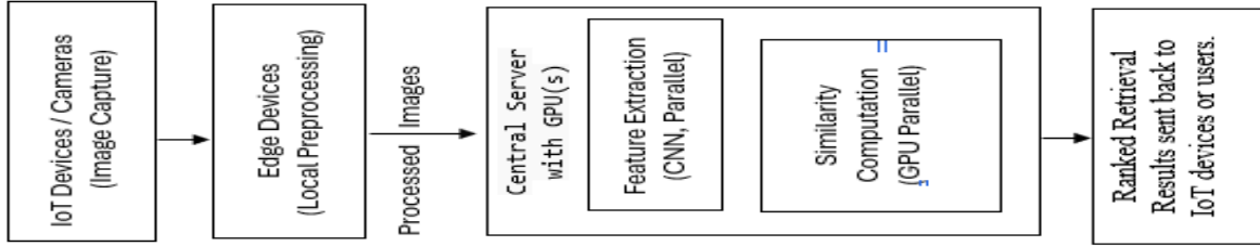
Figure 8. GPU-parallelized CBIR workflow in IoT.
