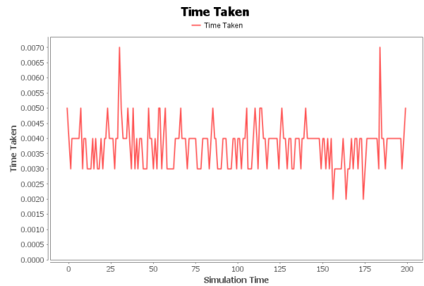
Figure 3. The time taken for the algorithm to calculate the jammer-angle assignments, in seconds
