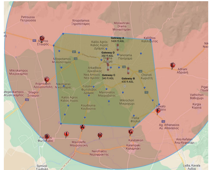
Figure 4. The 4 gateways along with the 27 test spots (blue pushpins) and 9 rural test spots (red push pins)
