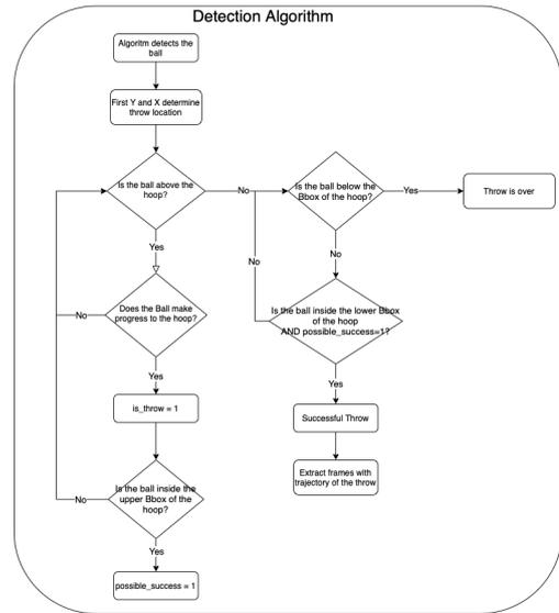
**Fig. 17.** Shot detection algorithm process
