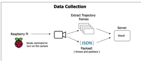
Fig. 9. Process and components of the system
