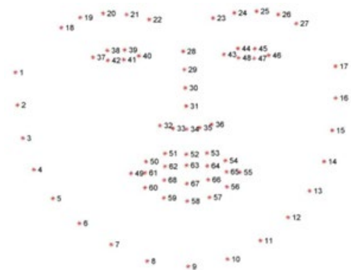
Figure 5. Facial Landmarks detected through Dlib
