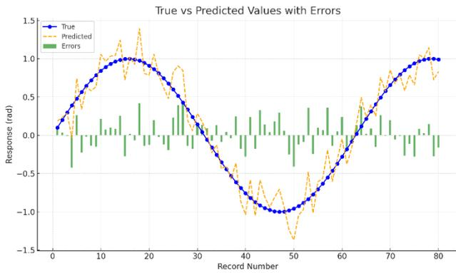
**Figure 6.** Analysis of performance for the Linear Quadratic Regression Model for Synchronisation Error in Node A and B.
