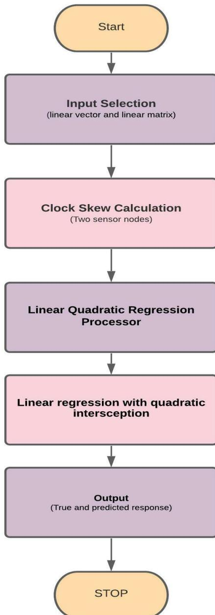
**Figure 5.** Proposed clock skew estimator using linear quadratic regression can be visually represented through a flowchart
