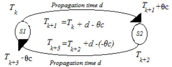
Figure 1. Bi-directional Message Exchange Scheme with Propagation Time and Clock Offset between S1 and S2.
