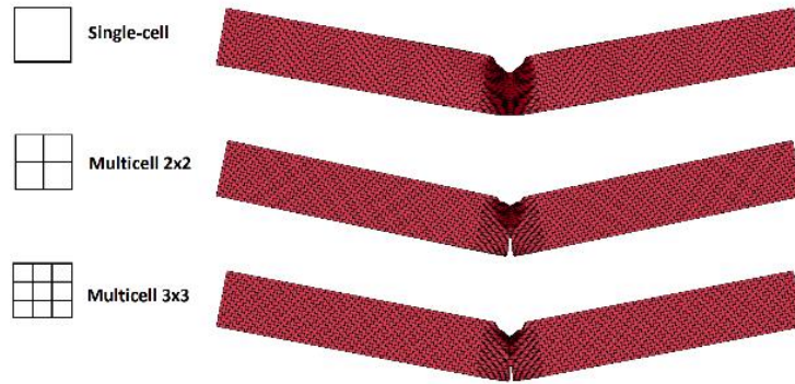
Fig 13. Deformation pattern of single-cell and multi-cell
