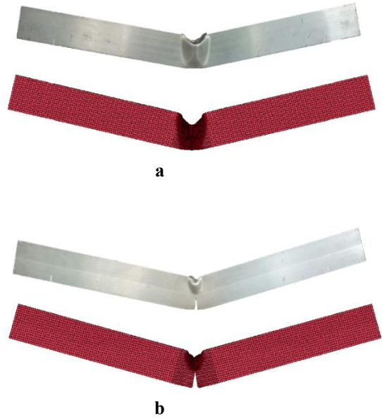
Fig 3. Experiment and Numeric deformation pattern a) Single-Cell b) Multi-Cell 2x2
