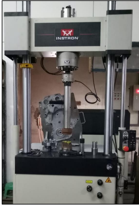
Fig 2. Quasi-static compression testing machine
