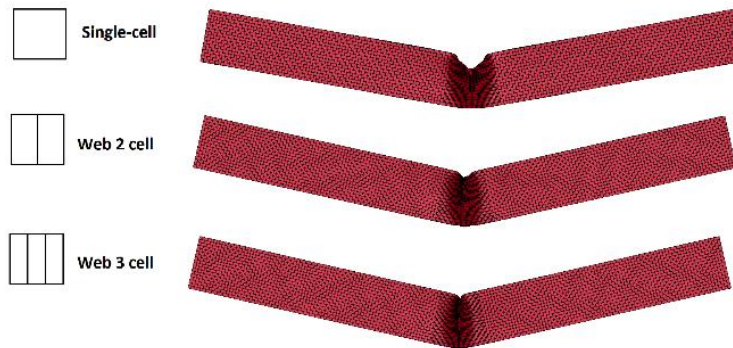
Fig 9. Deformation pattern of single-cell and web-cell
