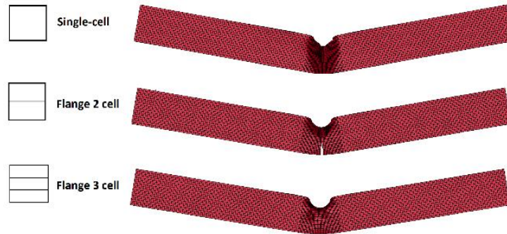
Fig 11. Deformation pattern of single-cell and flange-cell
