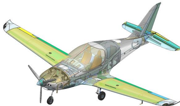
Fig. 7. URC-X01 electric aircraft configuration design
