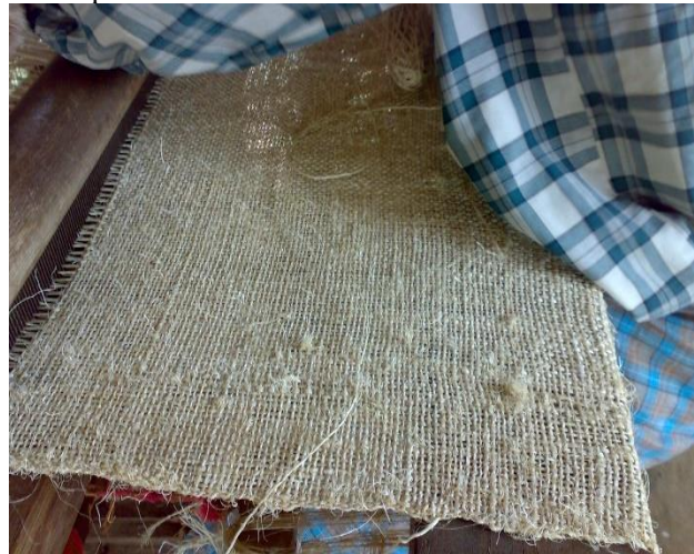
Fig.6. Agave fibers made into Fabric
