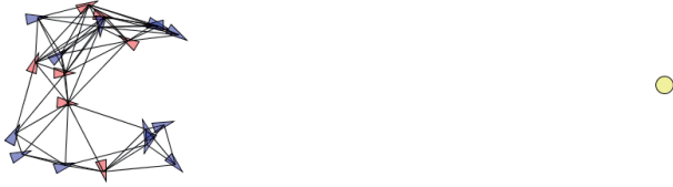
Figure 4: Beginning of the simulation: The flock is unstable. There are many leaders in a flock and the direction of movement is not decided yet. Red: leadership value \alpha \geq 0.5 (= leader ) , Blue: leadership value \alpha < 0.5 (follower), Link: interaction between boids
