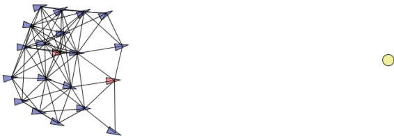
Figure 5: Last stage of the situation: The flock is stable. After the consensus of the direction of movement, the number of leaders becomes small. Red: leadership value \alpha \geq 0.5 (= leader ) , Blue: leadership value \alpha < 0.5 (follower), Link: interaction between boids
