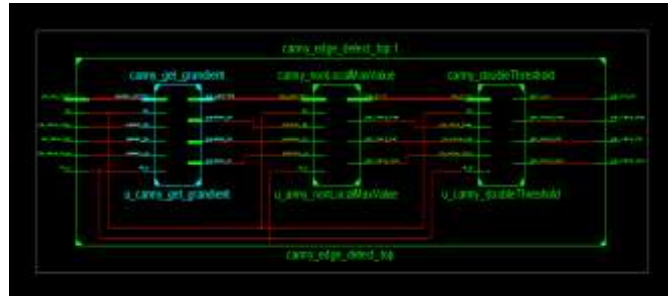
Fig. 18. Schematic Diagram of Proposed Canny Edge RTL design.
