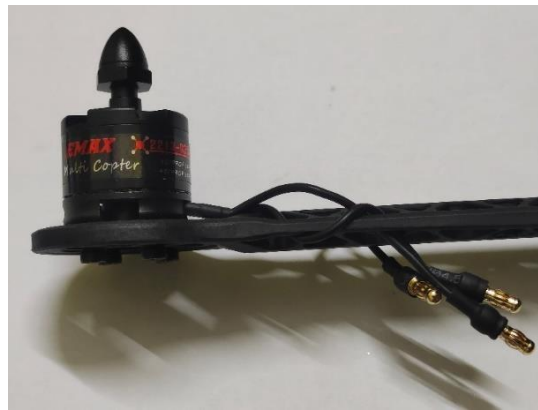
Fig.1. EMAX 935KV Brushless motor.
