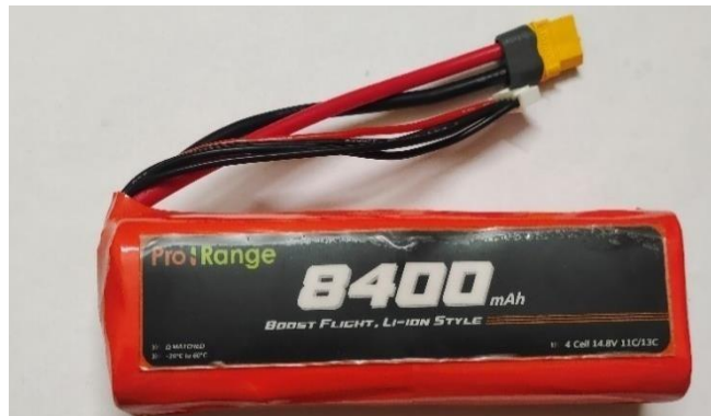
Fig. 7. 8400mAh 4S2P Li-ion Drone Battery.
