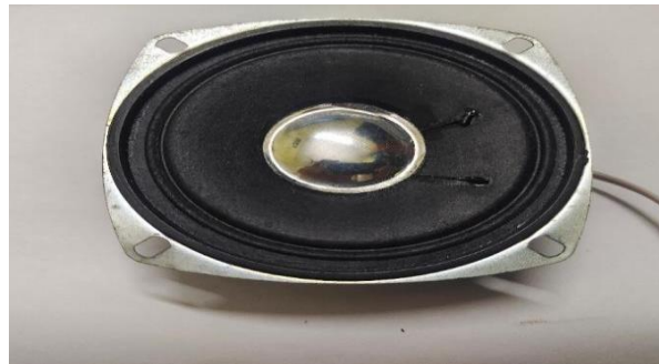
Fig. 11. 4-Ohm, 5-Watt Satellite Speaker.
