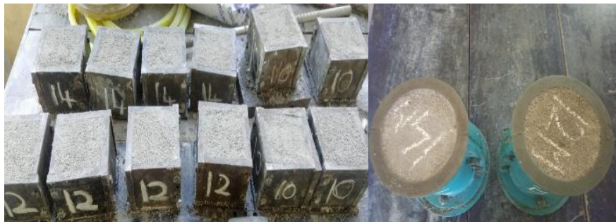
Fig. 4. Casting of Mortar Cubes and Cylinders
