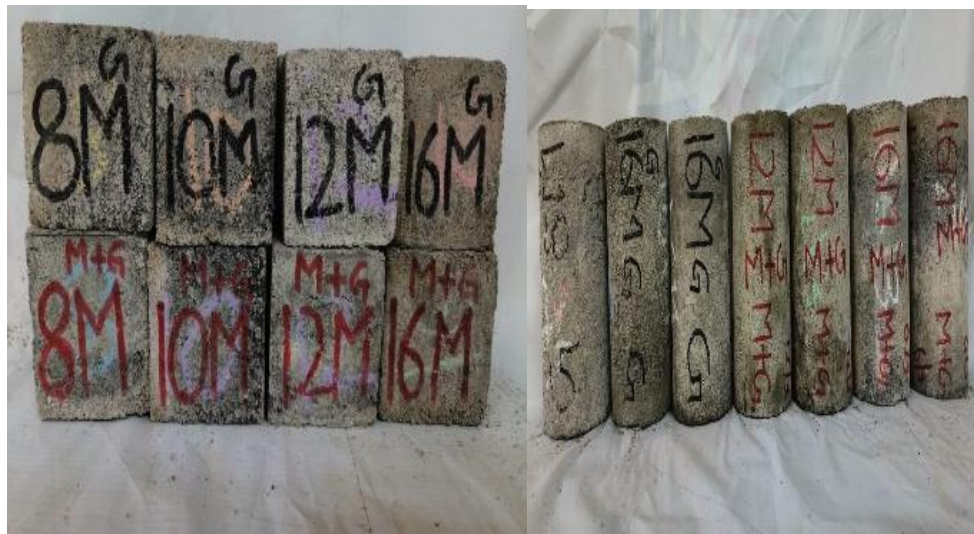
Fig. 2. Geopolymer Mortar Cubes and Cylinders of Different Molarities.
