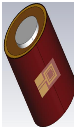
Figure 3. The RF sensor is mounted on the Bone tissues.
