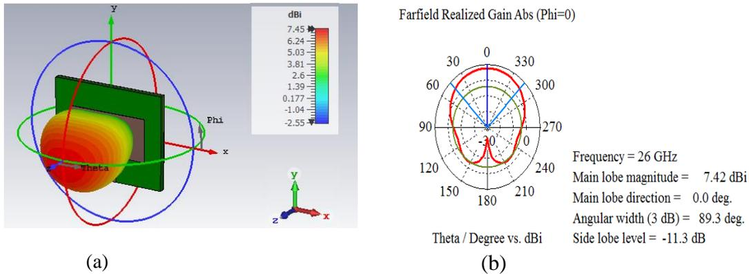
**Fig. 4.** Far field of the proposed inset fed patch antenna (a) 2D and (b) 3D
