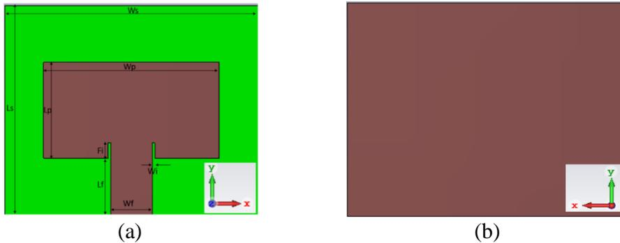
**Fig.1.** Geometry of the Proposed inset fed patch antenna (a) front view and (b) back view.
