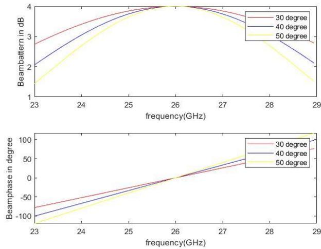
**Fig.6.** Magnitude and phase of the gain function with frequency at different incident angles.
