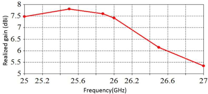
**Fig.3.** Realized gain vs frequency plot of the proposed inset fed patch antenna.
