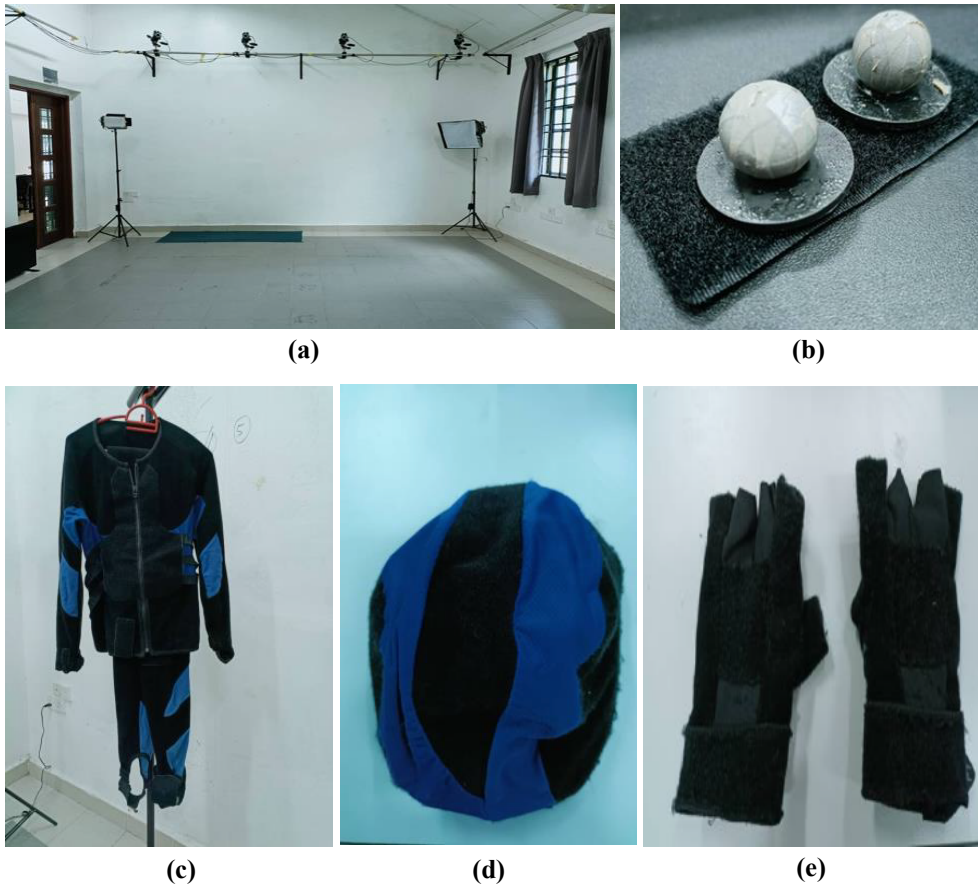
Fig. 2.: (a) Motion Capture space that equipped with 8 units infra-red camera of inertial measurement units (IMUs), (b) Marker Reflector indicator, (c) Motion Capture suit made of polyproline, (d) Head Cap & (e) a pair hand gloves (Resource: Researcher)
