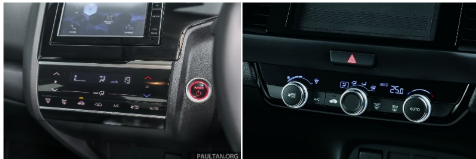
Fig 7. 2015 Honda Jazz (Left) and 2020 Honda Jazz (Right) Air Conditioning Controller
