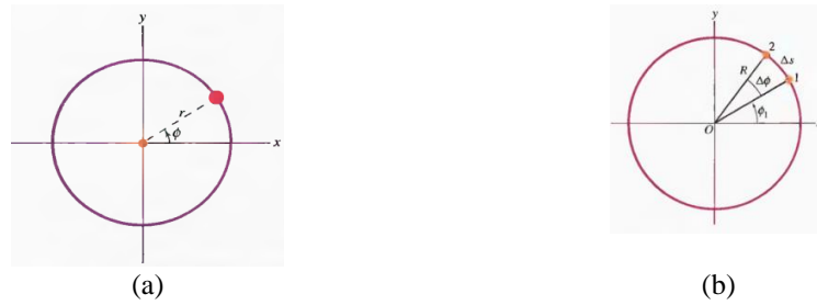
Fig. 2. (a) Radial variable r and angular variable \theta of plane polar coordinates. (b) During the time interval \Delta t a particle in circular motion transverses an arc length \Delta s and an angle \Delta\theta [6]
