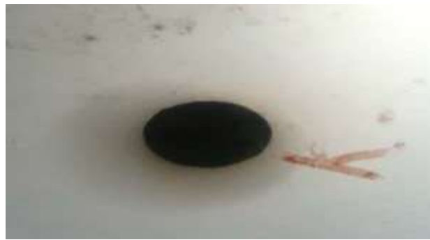
Fig. 15. Control plate with no thermal diffusion process (SS316L)
