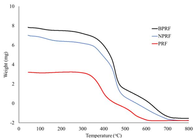
**Fig. 3.** TGA Curves of treated and untreated *P. ritcheyi* fibres
