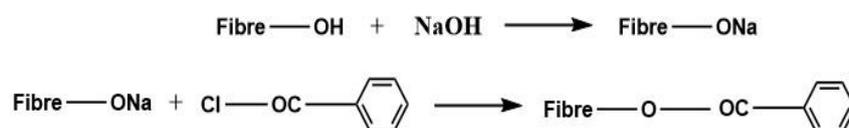
**Fig.1.**Fibre modification by benzylation treatment
