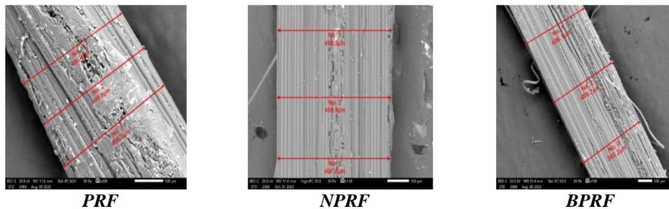
**Fig. 2.** Measurement of fiber diameter using SEM images.
