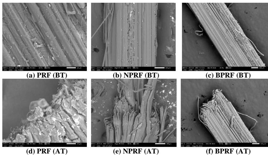
**Fig. 4.** SEM images of chemically treated single *P. ritcheyi* bamboo fibers: Before (BT) and after (AT) tensile testing.
