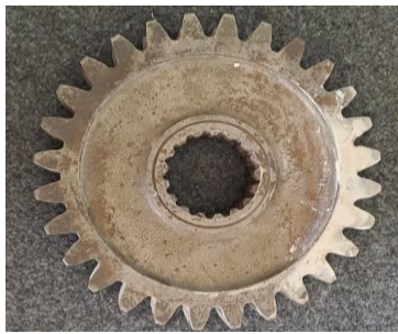
Figure 11. Repaired gear by Wire arc additive manufacturing with B07 as desired parameter
