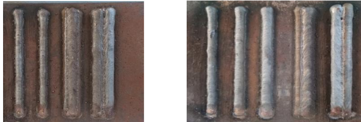
Figure 3. Single track deposition on substrate
