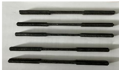
Figure 4. Specimen beads for tensile testing
