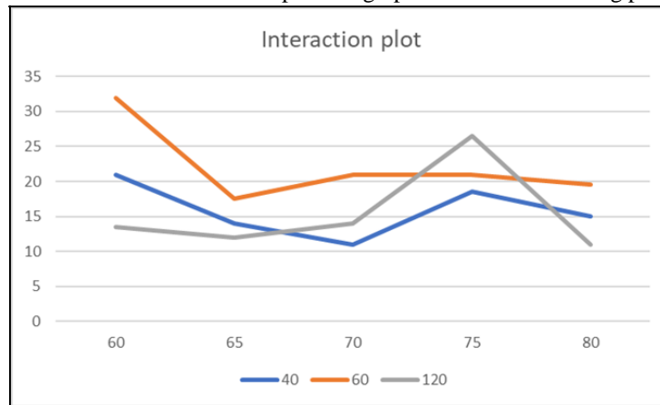
Fig 5. Interaction plot between bed temperature ( ^{\circ}\text{C} ) and print speed (mm/sec)
