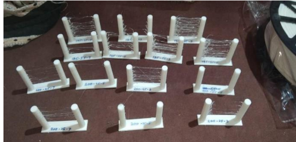
Fig. 2. Formation of Strings in fabricated specimens using Ender 3 Printer
