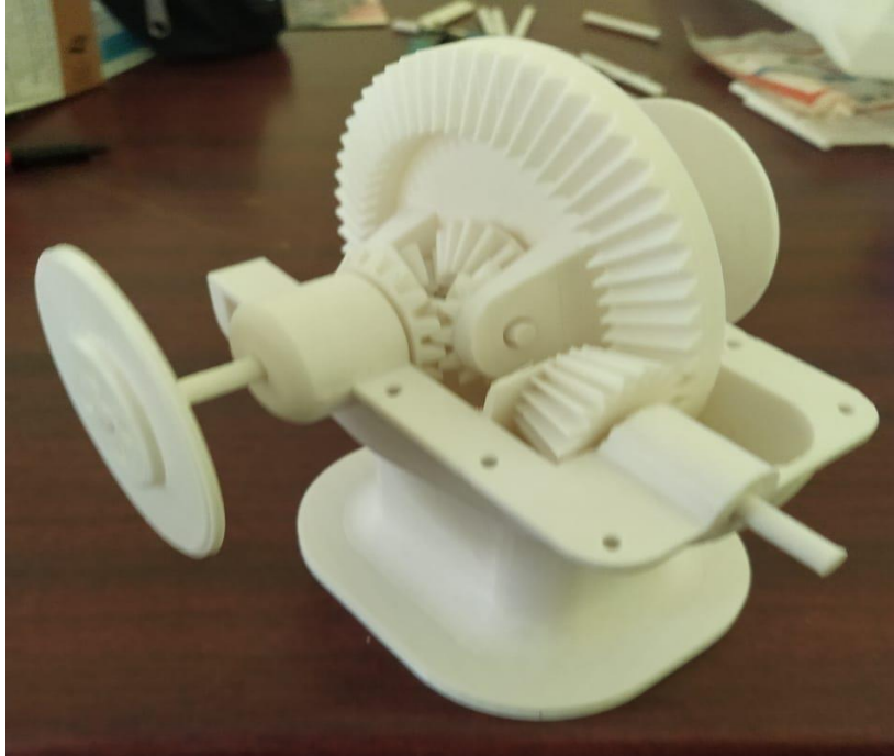
Fig. 9 Fabricated differential gear model.
