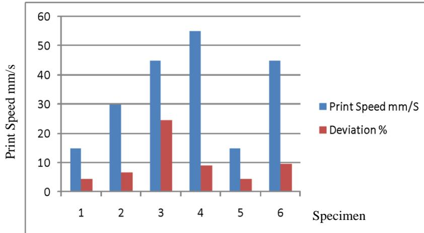
**Fig. 3.** Effect of Print Speed on Deviation Specimens 1,2,3,4,5 and 6
