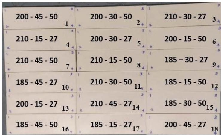
**Fig. 2.** FDM Fabricated Parts
