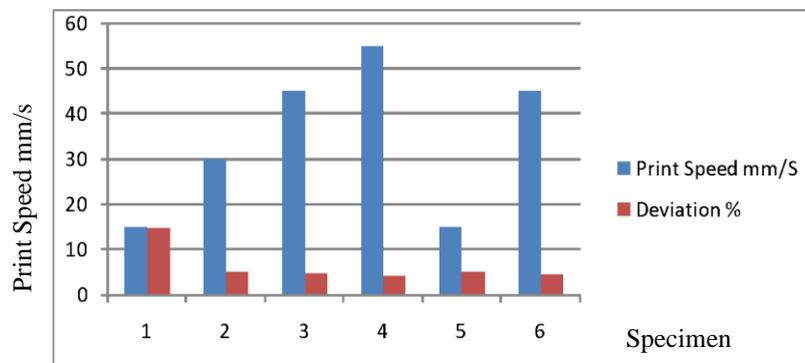
**Fig. 5.** Effect of Print Speed on Deviation Specimens 13, 14, 15, 16, 17, and 18
