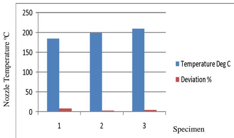
**Fig. 6.** Effect of Nozzle Temperature on Deviation Specimens 6, 12 and 18
