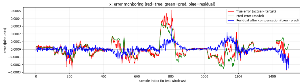
Fig. 5. Error compensation results in the X dimension (Picture credit: Original)
