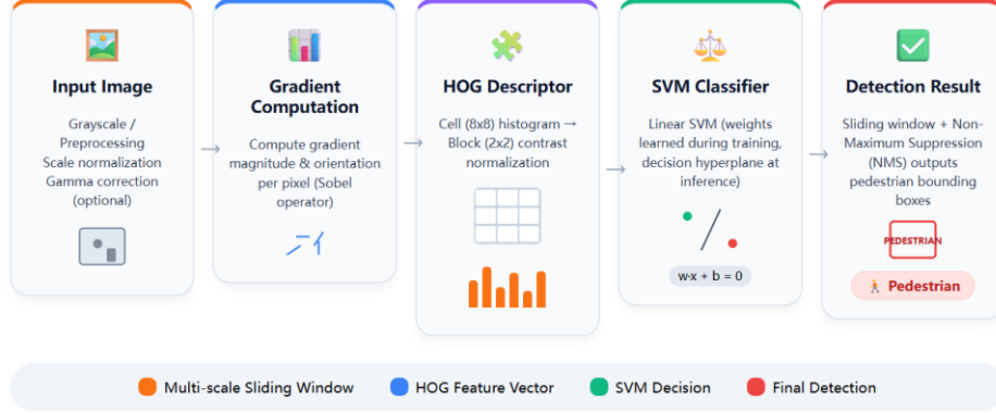
Fig. 1. Flow diagram of pedestrian checking through HOG+SVM (Picture credit: Original)
