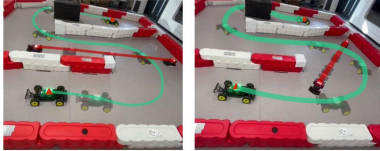
Fig. 3. A F1TENTH vehicle navigating through dynamic environments using the RSTP method. Green denotes vehicle trajectory, while red denotes the trajectory of dynamic obstacle [9].
