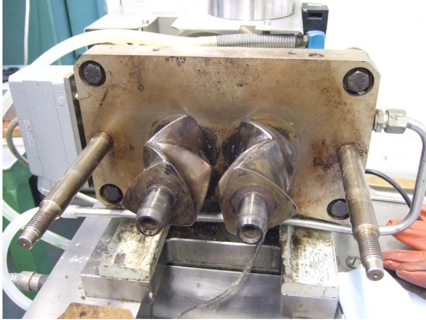
Fig.4. Homogenization of recycled polyvinyl butyral by Brabender Plasti-Corder W 350 E[12]
