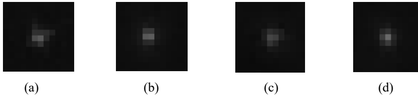
Fig. 2. Local star points of the star map under 1°/s dynamic after denoising by different methods: (a) Real star map local star points; (b) Local star points of the star map after denoising with GATFP [19]; (c) Local star points of the star map after denoising with Open Operation [20]; (d) Local star points of the star map after denoising with DSR-Net.
