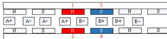
Fig. 1. permanent magnet synchronous linear motor cycle topology.
