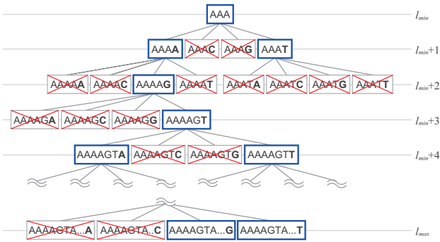
Figure 2. Outline of ORS estimation with reducing the search space. The strings in blue rectangles and red crosses are selected and excluded, respectively. Z -scores between parent and child nodes are compared, and if Z -score of the child node is smaller than that of the parent node, the sequence on the child node is excluded.
