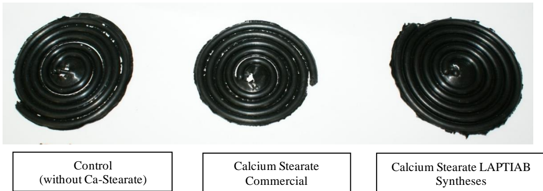
Fig 4. Rubber Molding Product Using Rubber Processing Aid (RPA) of Palm Based Calcium Salt
