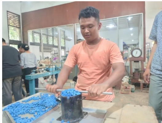
Fig. 4. Bulk Density Test on plastic aggregates
