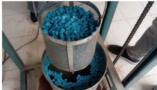
Fig. 7. Floating AP1 sample in specific gravity and absorbion test
