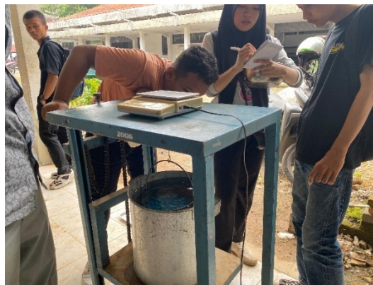
Fig. 6. Specific Gravity Test on plastic aggregates.
