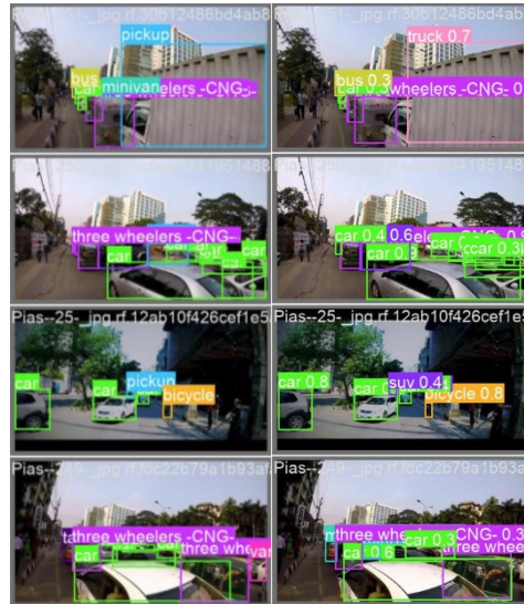
Fig. 1. Anchor Box Comparison ( Image on the left side: Real Anchor Boxes; Image on the right side: Ultralytics/YOLOv5).
