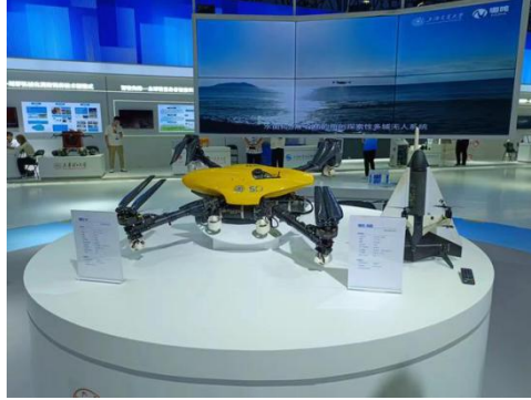
Fig. 4. The “Nezha” sea-air integrated cross-domain vehicle platform developed by Shanghai Jiao Tong University
