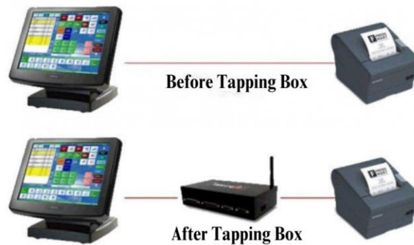
Fig. 1. Before and After Installing the Tapping Box on the Cash Register
