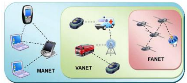
Figure 4. Architecture of MANET, VANET and FANET [10]
