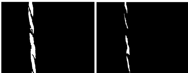
Figure 15. Results obtained from the application of the algorithm: (a) Application of the Otsu algorithm for segmentation.; (b) Application of a morphological erosion operation.
