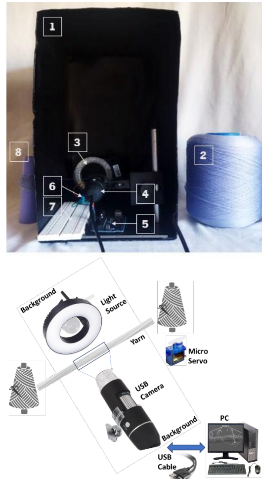
Figure 3. Prototype of the image acquisition system (left), and schematic diagram illustrating the component layout and acquisition geometry (right).
