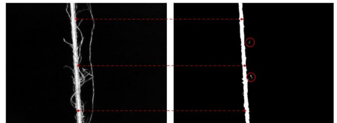
Figure 19. Result of the individualization of the core of sample B226.
