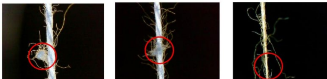
Figure 21. Some of the defects identified: (a) Nep identified in sample A91; (b) Thick place identified in sample A406; (c) Thin place identified in sample B301.
