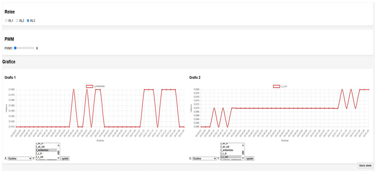
Figure 6. Web interface module for advanced dynamic control, including relay management and PWM
