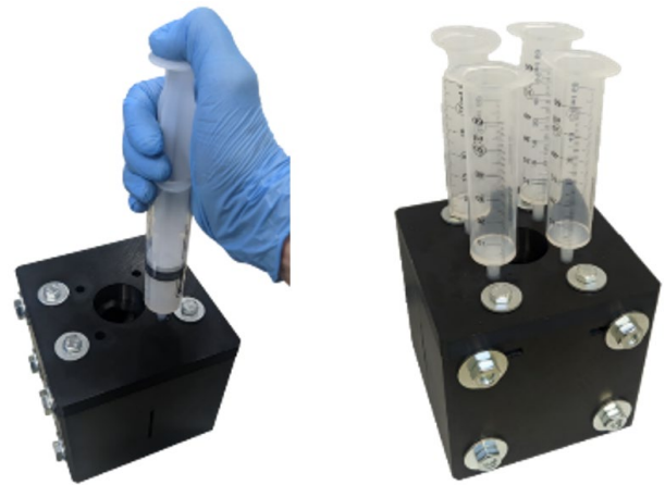
Figure 9. Process of filling the casting mold
