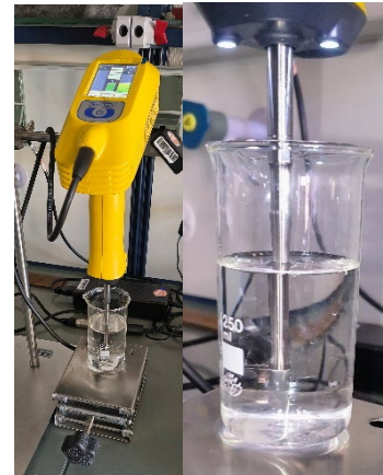
Figure 1: UP200Ht and sonotrode S26d7
