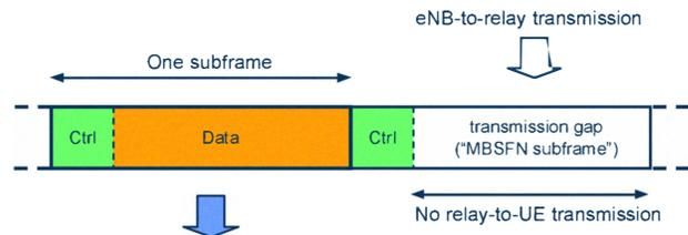
Figure 2. MBSFN and normal subframes for relay-UE link.
