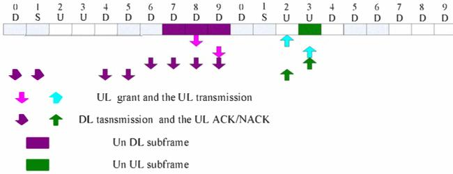
Figure 8. Un subframe allocation for DL-UL Config #4
