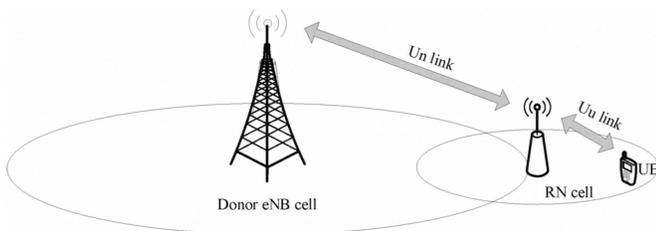
Figure 1. Backhaul (Un) link and access (Uu) link in a two-hop relay.
