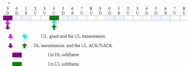
Figure 10. UL subframe allocation DL-UL Config #6
