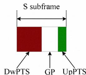
**Figure 3.** Structure of S subframe in TDD LTE[5].
