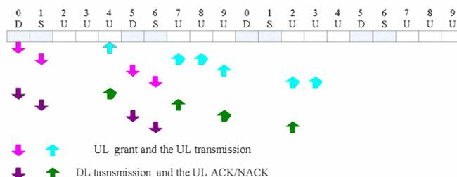
**Figure 4. Un subframe allocation for DL-UL Config #0**
