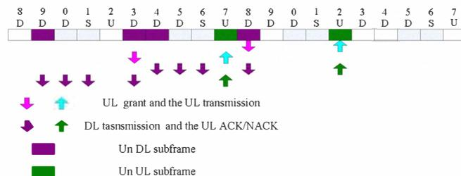
Figure 6. Un subframe allocation for DL-UL Config #2
