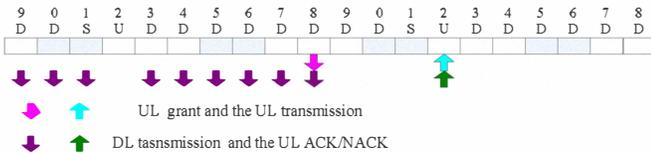
Figure 9. Un subframe allocation for DL-UL Config #5
