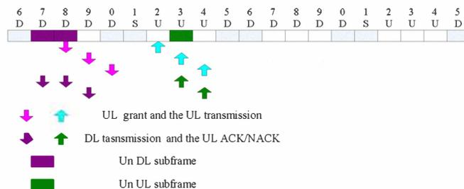
Figure 7. Un subframe allocation for DL-UL Config #3
