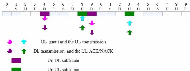
Figure 5. Un subframe allocation for DL-UL Config #1
